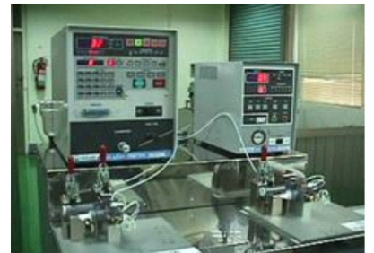
Pressure Leakage Testing Equipment
