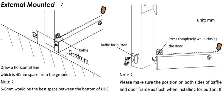
to the ground. If the door gap is too big then 40mm space remaining between the top of DDS to the ground would be the best. (Draw a horizontal line which is 40mm space from the ground before install). Please make sure the position on both sides of baffle and door frame as flush when installing for button. If gap exist between door and door frame, please adjust the distance for baffle and DDS to make sure the adjustable button can be pressed completely without gap while closing the door.
