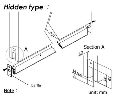
Install the adjustment on the rotatable side of door end. Make the bottom groove<sup>1</sup> according to "section A" and cut the DDS with suitable width<sup>2</sup> for door. Install DDS into the groove and fasten the baffles on both sides of the door.
